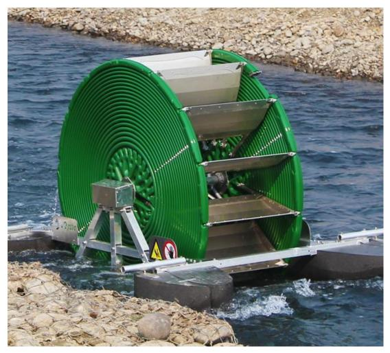
Fig 2: Barsha Water Pump Source: aQysta Company
