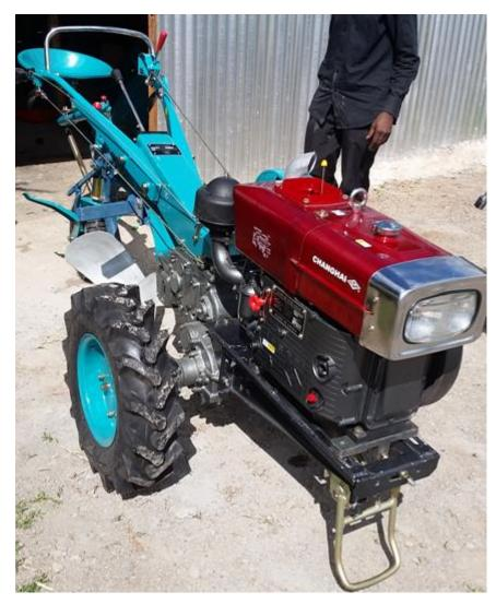
Fig 14: Single Axle Tractor Source: Greentree
