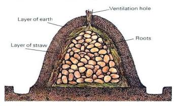
Fig 20: Clamps Source: Kale et al,2016
