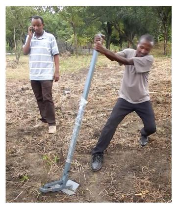
Fig 8: Tree Puller Source: water channel
