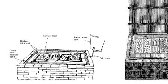
*Fig 18: Static cooling chamber source: Practical Action*
